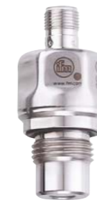
Pressure sensor type PL15 1/2" ceramic measuring cell. 2/3-wire selection. Medium temperature transmission via IO-Link.
